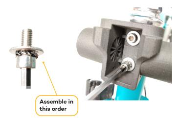
2 Attach the Quick Connect Handlebar Mount to the adapter. Don't use the spacers or the twist strap.
