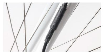
8 Ensure the motor is fully connected – hear the "click" To connect the waterproof connector, align the arrows and push together until the arrow on the motor wire connector is touching the Mount connector. The photo below is not properly connected.
