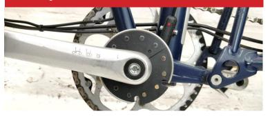
**BROMPTON INCORRECT MOUNTING METHODS** Mounted onto correct tube but gap is too big
