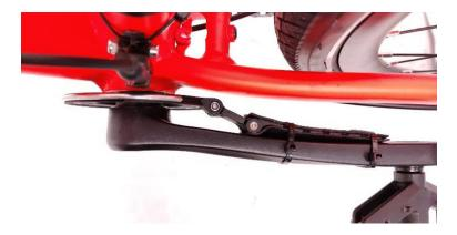
Loosely cable tie the magnet disk arm to the inside of your pedal arm in at least 2 points. Reposition the magnet disk so that it is close to the sensor and aligned. Check that the alignment is correct by rotating the pedal arm backwards and watching for any movement. After this check, tighten the cable ties completely.
