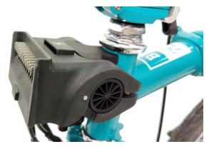
3 Connect your Pedal Sensor, Brake Sensors and Throttle to the bracket. You will need to use extension cables to reach the new position.
