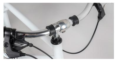
**Place mount onto handlebars angled upwards 45°** Fit the Quick Connect Handlebar Mount over the spacers onto the handlebar, then rotate the mount to 45°.
