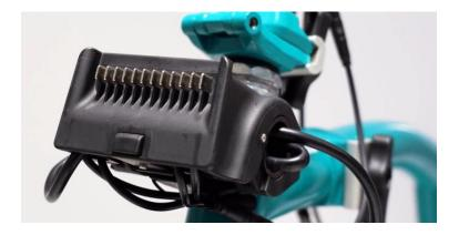
8 Secure the cables underneath the bracket with a cable tie threaded through the hole in the bottom.
