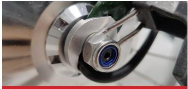
Be careful not to damage the motor cable when tightening the nut
