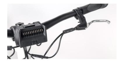
You can also assemble the brake sensors onto any point along the brake cable.
