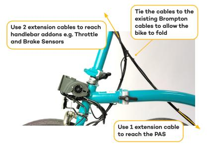
Shorten the motor cable by folding it back on itself and securing it with a cable tie. Make the loop the same length as the length of the Brompton Block Adapter.
