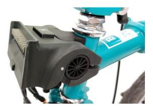
The Bro Block Adapter allows the Power Pack to be mounted directly to the frame.
