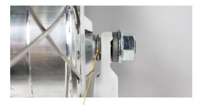
Add spacers if the motor casing touches the forks
