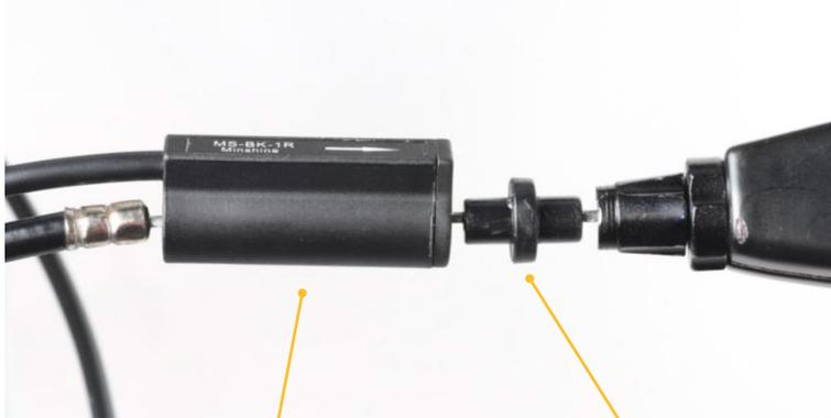
Brake sensor goes "in line" with the brake cable, which is fed through it
