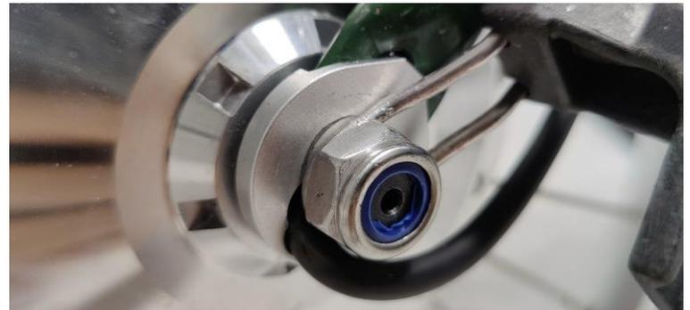
Be careful not to damage the motor cable when tightening the nut
