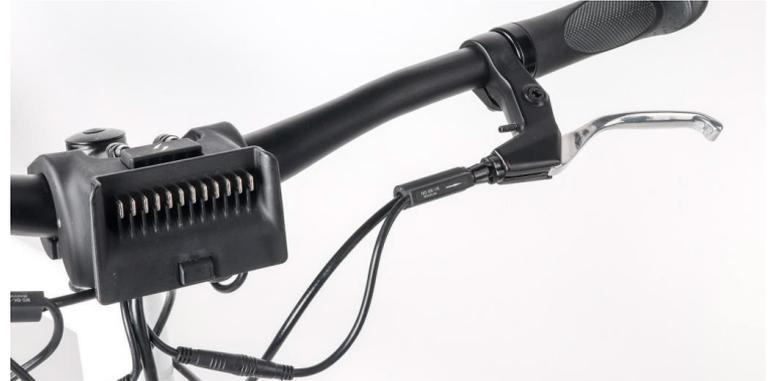
You can also assemble the brake sensors onto any point along the brake cable.
