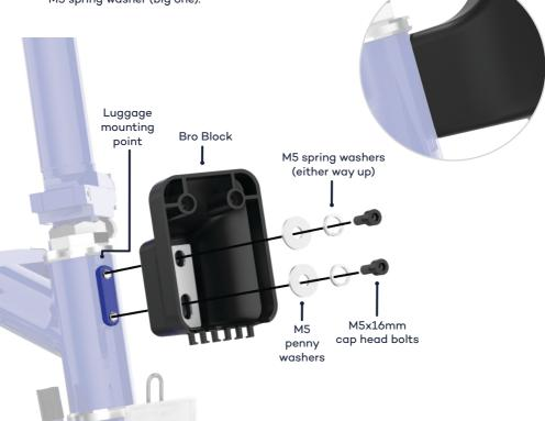
The graphic above shows the parts for a Brompton bike installation.
