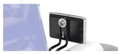
1.2 Align the reflector and then retighten the screw to secure it in place.
