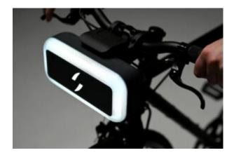
The most visible change is that the front of the power pack now sports a ring light. This is billed as an "omni-direction be-seen light" so it's a visibility feature really. There's also a USB-C port on the back, so you can charge your phone from it.
