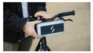
The new range-topping Max++ <u>ebike conversion kit</u> uses a case design that fits more cells than ever. The battery capacity is upped to 370Wh, putting it on a par with lightweight ebike systems such as Mahle's X20, found on electric road bikes including BMC's Roadmachine AMP. The Max+ has a 280Wh battery with a claimed range of 20 to 40 miles, a step up from the basic Air and Go systems (90Wh & 180Wh respectively).
