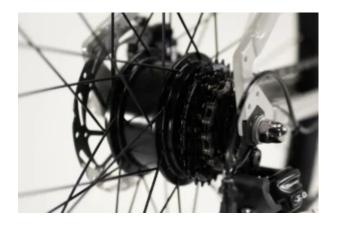
Swytch is also now offering Swytch kits with a rear-hub motor. The new rear hub can be supplied with either a standard or thru-axle and is compatible with both rim-brake and disc-brake bikes. The rear motor also includes an integrated pedal sensor.
